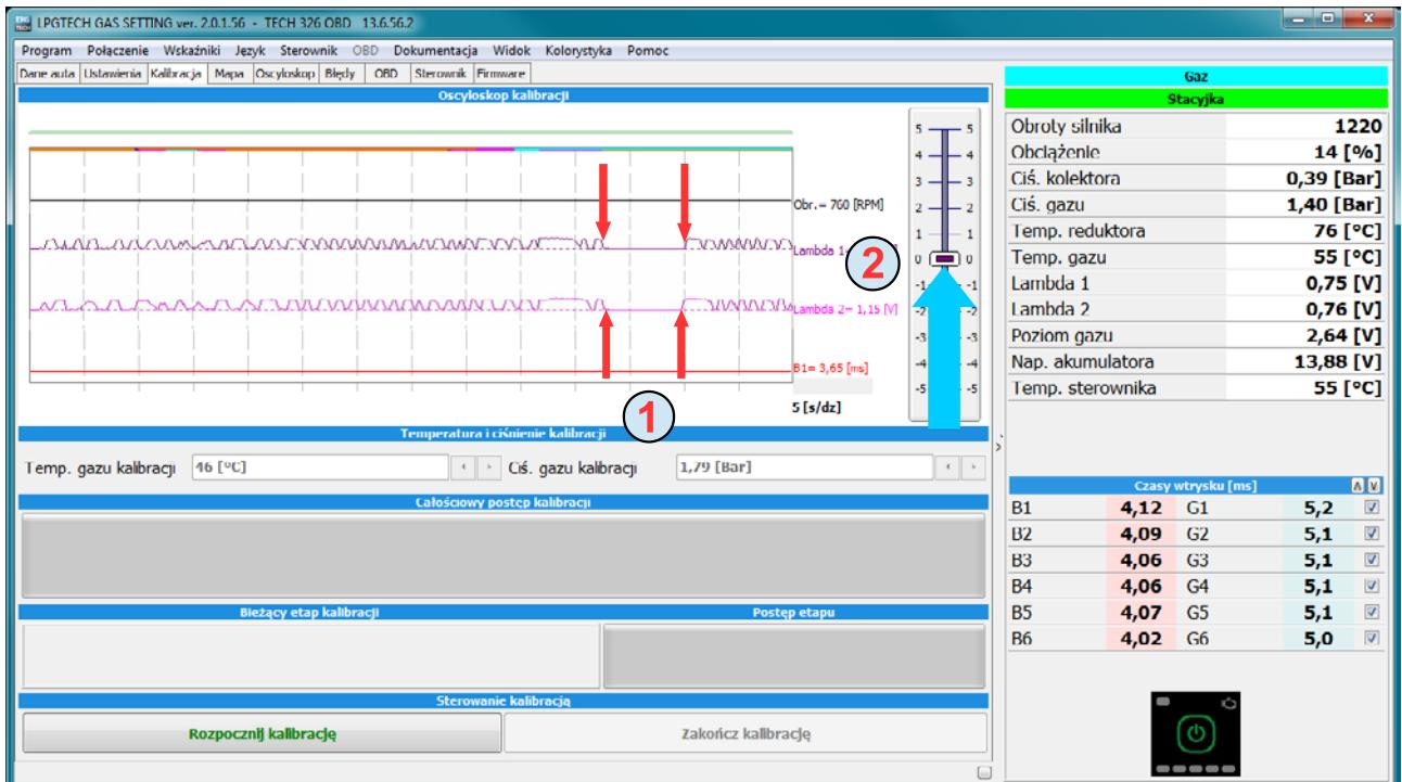
Img. 12. Example overlooking oscillating lambda sensors
